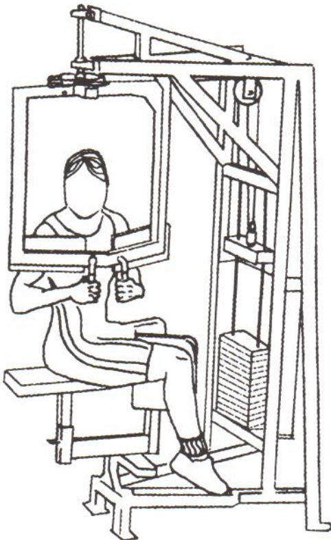
Fig. 1. The trunk rotation training machine ("Torso Trainer") used for the dynamic abdominal training program.
