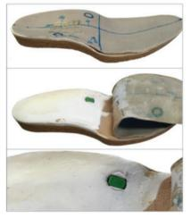
Fig. 1. Custom-made inlay with built-in sensor.
