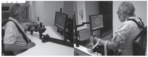
*Fig. 1.* The two InMotion® (Interactive Motion Technologies, Waterown, USA) upper extremity robotic units used in this study. (A) The proximal unit providing repetitive movements to the shoulder and elbow joints. (B) The wrist unit focusing on the wrist joint.
