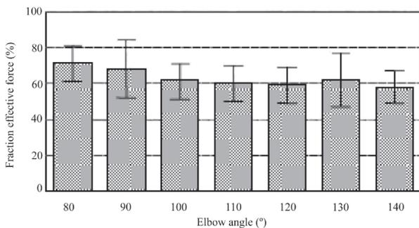
Fig. 3. Mean (standard deviation) fraction effective force for 12 subjects with a spinal cord injury at different seat heights (80–140°).
