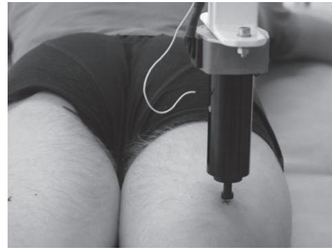
Fig. 1. Direct measurement of muscle tone with computerized tonometer. The motor pushes the indenter at a constant speed onto the muscle and resisting force and travel are registered continuously. The work performed is calculated from these parameters.
