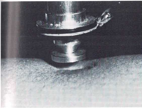
Fig. 1. Oedematous tissue was compressed for 20 sec by a cylindrical head 15 mm in diameter to a depth of 4 mm. After withdrawal of the compression head, a depression remained due to the translocation of oedematous fluid.
