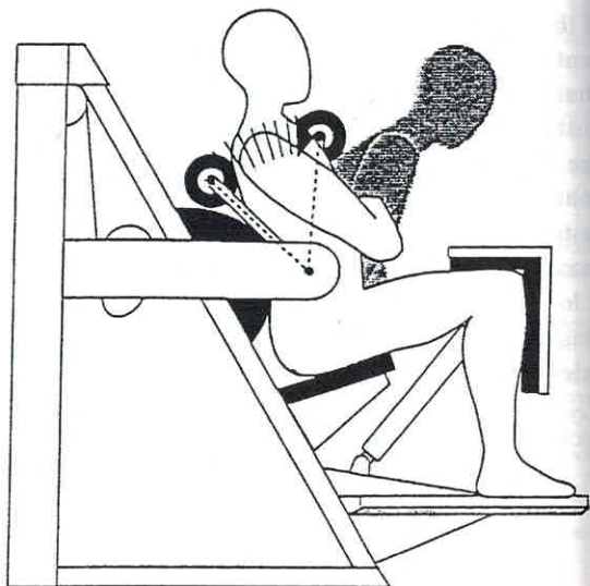
Fig. 1. The DBC 110 testing and training device. The fixation mechanism for hip, knees and feet was adjusted in such a way that the vertebral columns below L3 level were guided not to move. A cam mechanism created a variable resistance pattern (isoinertial movement) along the movement range which was adjusted between 25° flexion and 5° extension.
