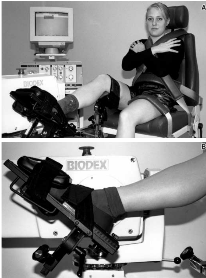
Fig. 1A, B. Illustrations showing the positioning in the Biodex dynamometer for measuring isokinetic ankle dorsiflexor strength.
