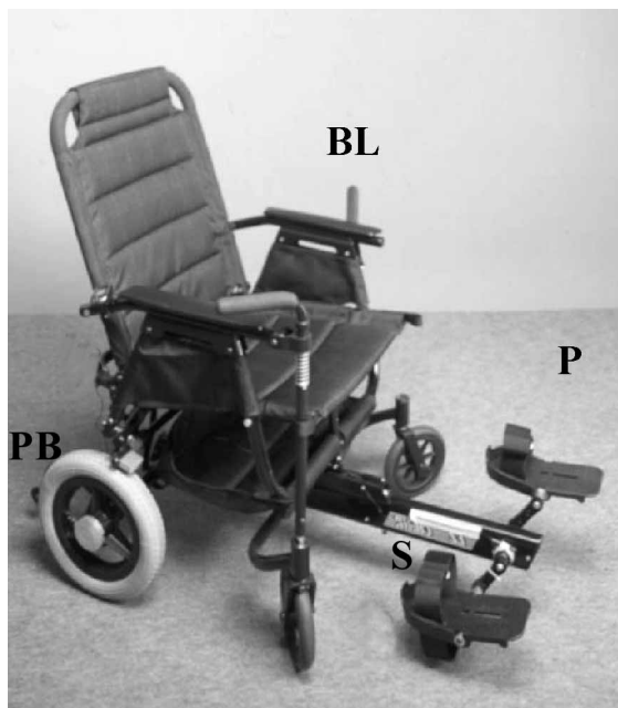
Fig. 1. Leg-pedalling wheelchair for a left hemiplegic patient (EZchair ® ). PB = parking brake; BL = brake lever; S = shaft connecting the pedals and wheelchair; P = pedals.
