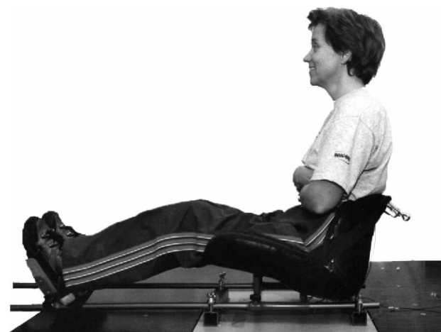
Fig. 1. The experimental set-up for balance testing. The subject is sitting in a special chair which is also used in the kayak. The chair is firmly attached to a force plate. The subject's feet are resting on a support connected to the chair via steel rods.
