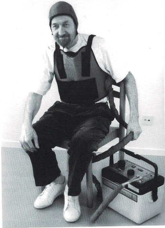
Fig. 1. The cooling suit comprises a vest and a head cap, with channels for circulating cooling fluid, attached to a cooling box (Mark VII Microclimate Cooling suit, Life Support Systems Inc., Mountain View, CA, USA).
