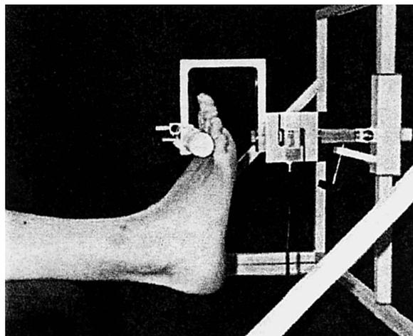
Isometric dorsiflexor torque measurement with the ankle in neutral position (0°). The plastic beam at the level of the metatarsalphalangeal joints is connected by a U-shaped hook to a load cell.
