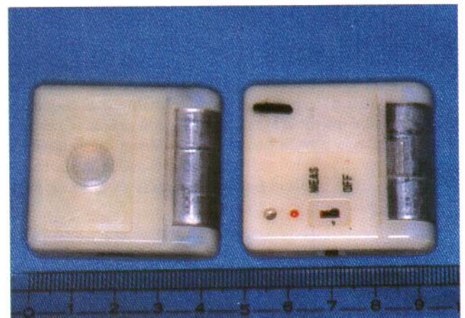
Fig. 1. The Scratch-Monitor (SM). The two SMs (the right one is No.1 and the left one is No.2) have the same structure. The switch button is on the upper side, and a button for the marker is on the left side. A pressure sensor is under the SM, by which the number of scratch movements is recorded if there are more than three consecutive changes in pressure at a rate of about once or more/second.
