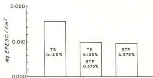
Fig. 34. Residual EPESC Levels After Simulated Dish Washing With TS, TS + STP, and STP Alone.
