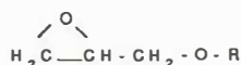
Epoxide 8 (glycidyl ether of aliphatic alcohols; R is predominantly a C 12 or C 14 alkyl chain)
